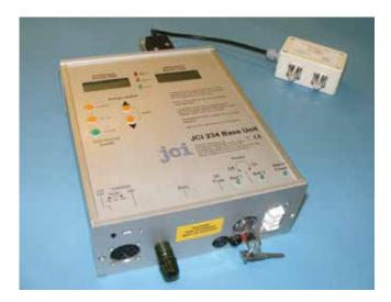
The JCI 234, in conjunction with the JCI 131F fast response fieldmeter, provides the ability to resolve and measure both quasicontinuous electric fields and superimposed 50/60 Hz alternating electric fields which are viewed on an additional display. The JCI 131 and JCI 234 can be operated from the separate mains input power supply or from a 12 V battery for uninterruptible power supply.
