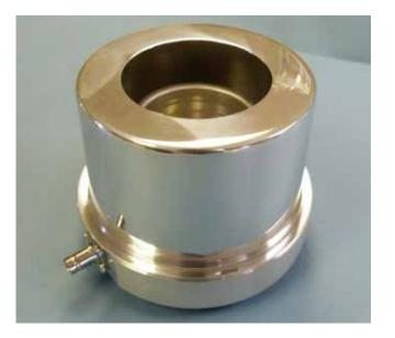
virtual earth charge measurement unit is made via cable connection to the BNC connector.
